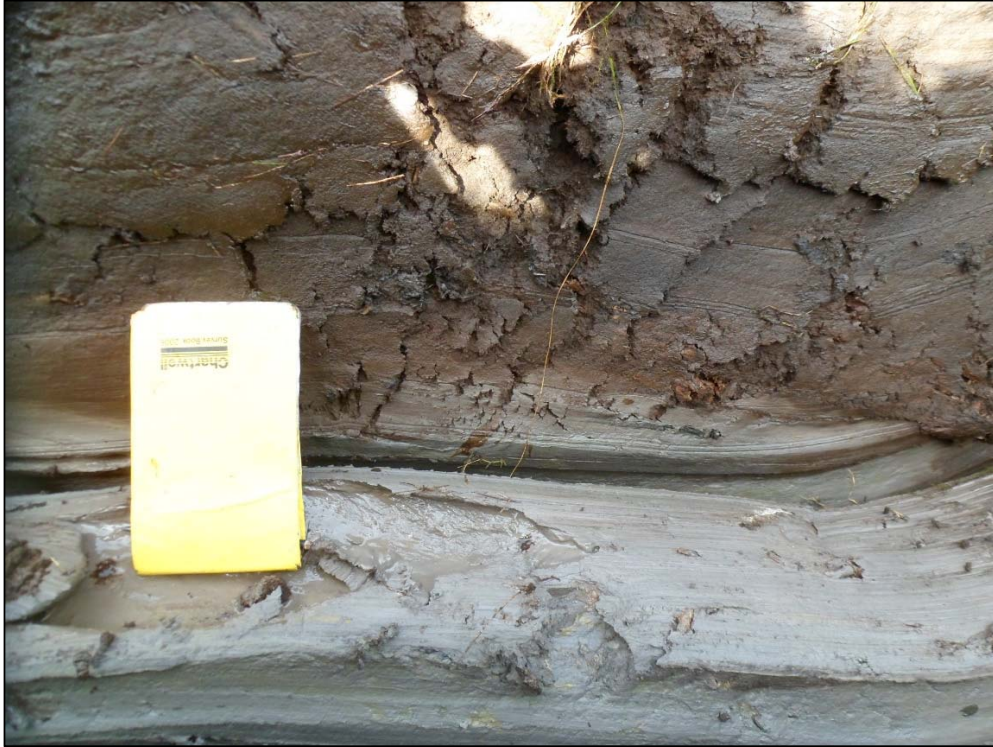
Photo 3 Underlying soft silt/clay at trial pit TP2
