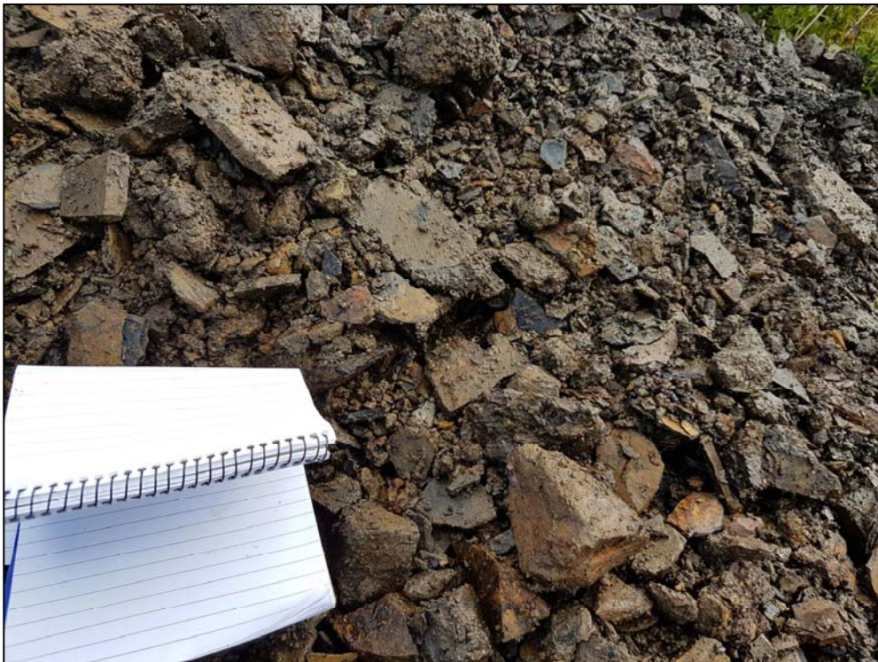
Photo 4 Example of shale rock present at proposed borrow pit
