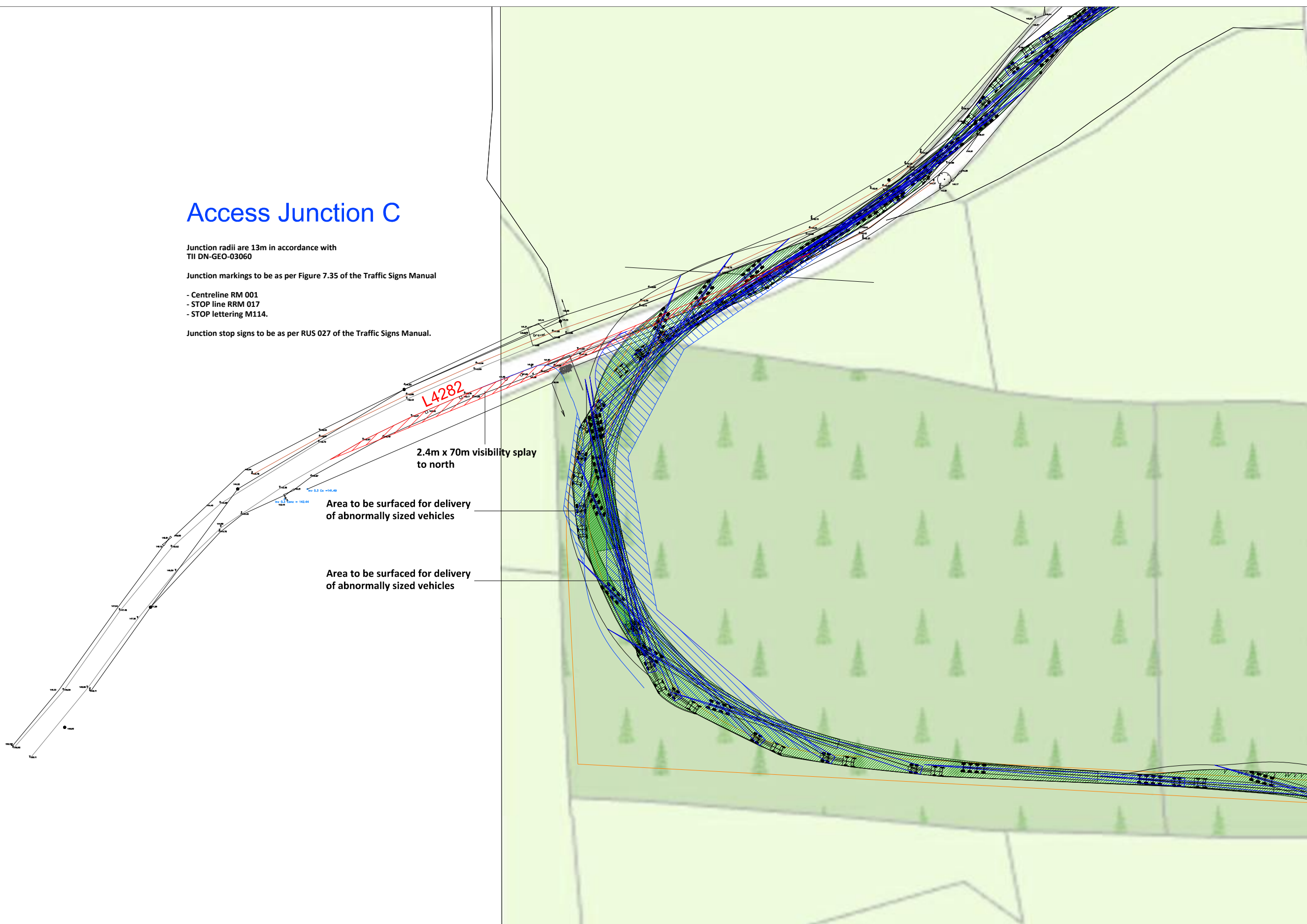
Figure 14.16 Location 5 - Access C - L4282 - Turbine access and general construction access, autotrack assessment for blade extended artic
