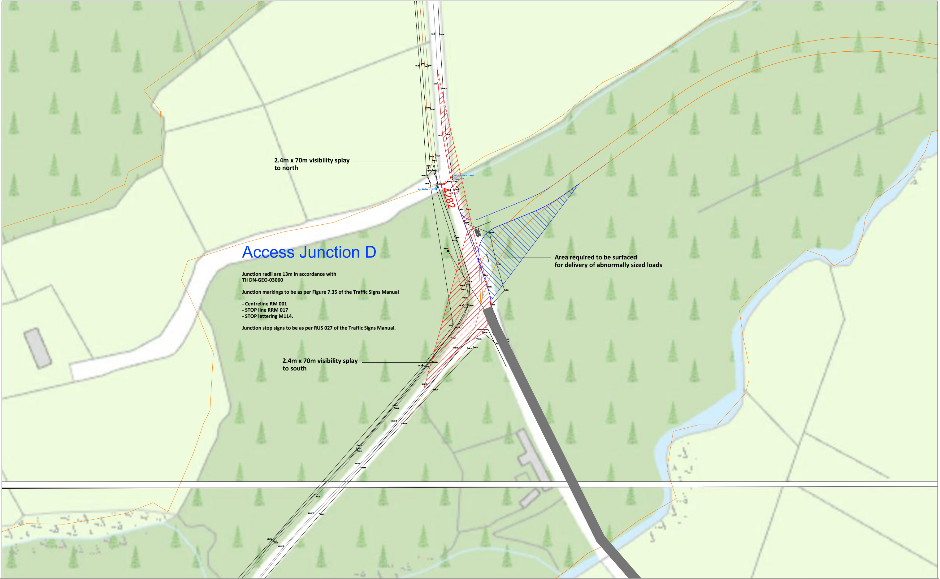
Figure 14.18 Location 6 - Access D - L4282 - Turbine access and general construction access, proposed layout and visibility splay
