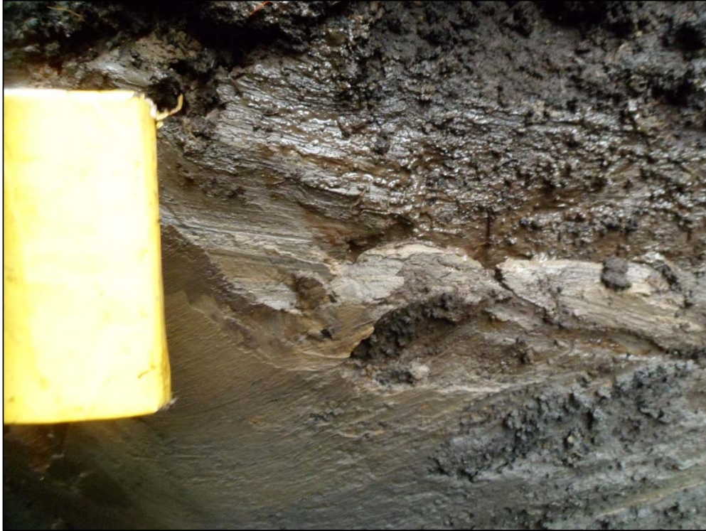
Photo 5 Underlying soft silt/clay at trial pit TP3
