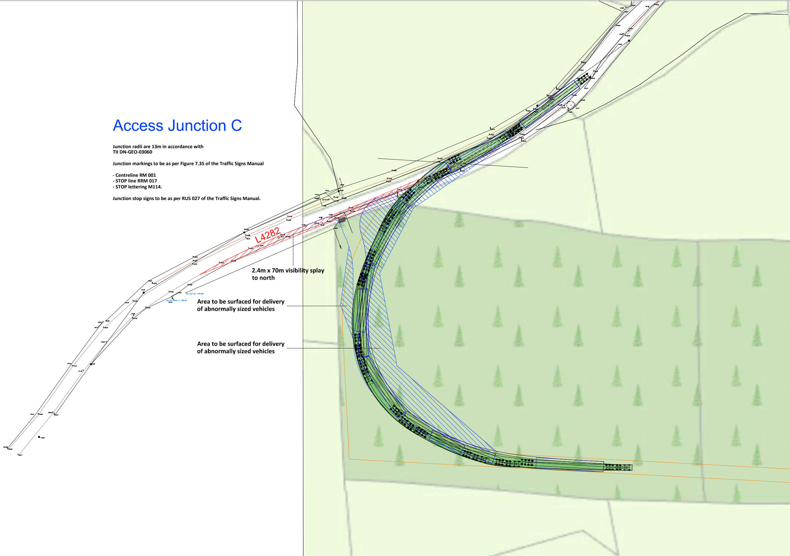
Figure 14.17 Location 5 - Access C - L4282 - Turbine access and general construction access, autotrack assessment for tower extended artic
